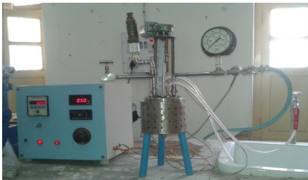
Fig. 4. Photograph of the assembled CSTR with connections to pressure gauge, temperature controller and pressure relief valve. The cooling coils are also used to control the temperature.
