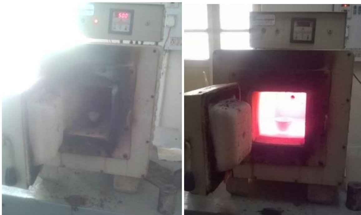
Fig. 6. 1 g of the residue heated to 500°C and 1000°C in a muffle furnace.
